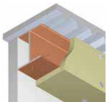
3 Two-sided protection with stud welded pins (up to 2 hours fire protection)
