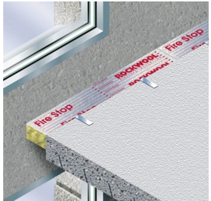
ROCKWOOL SP Firestop Slabs at floor / external wall junction, International Patent Application PCT/GB98/01733.
